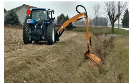
Boom Mower-Used for Mowing Areas Inaccessible by a regular mower for Ditches or Overpasses
